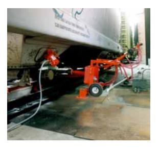
The Martin® Railcar Opener provides up to 2,500 foot pounds of torque to power open stubborn railcar gats.
