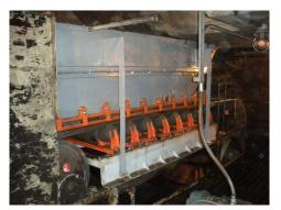
With the EVO® External Wear Liner installed, the plant can provide effective sealing of the belt edge with Martin® ApronSeal<sup>™</sup> Skirting.
