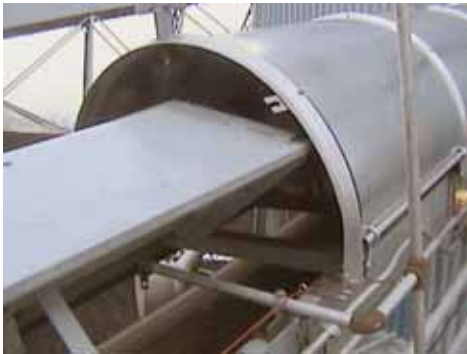
To allow installation of a belt scale for blending accuracy, the Martin® Air Supported Conveyor ties into a conventional roller-supported conveyor outside the transfer structure.
