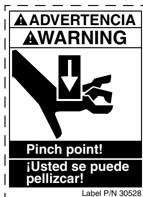
Figure 24. Pinch Point Warning Label, P/N 30528
