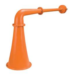
Martin® Sonic Horns generate and magnify low-frequency, high-pressure sound waves to cause dry particulate build-up to resonate and fluidize, allowing the material to be removed from the vessel by constant gas flow or gravity. The Martin® Sonic Horn 75 Hz 90 Degree produces 147 dB at one meter with a frequency of 75 Hz.
