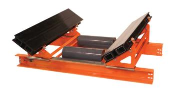
The **EVO**<sup>®</sup> **Slider Cradle** utilizes low friction UMHW bars to support the belt at the outside of the load-carrying area. This stabilizes the belt line, eliminating the sag and bounce that spill material, and reducing the risk of catching lumps that can abrade the belt surface.
