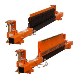
The Martin® SQC2S™ Cleaner incorporates individually-cushioned tungsten carbide blades for effective cleaning without risk to belt, splice, or blade. Installed in the secondary cleaner position, the Martin® SQC2S™ Cleaner's blade buffers cushion impact and maintains cleaning pressure.
