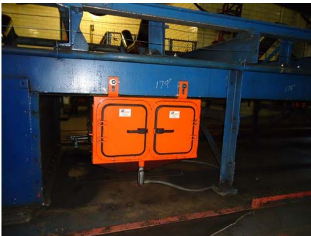
In a move designed to reduce maintenance and better control fugitive material, an innovative Michigan power supplier has installed customized wash boxes from Martin Engineering on its coal conveyor belts, slashing cleanup time while drastically reducing surface dust and airborne particles. Believed to be the first wash boxes used successfully on the tripper floor of a PRB
