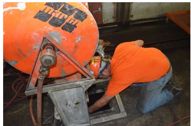
The Martin® Heavy Duty Whip is a portable, remote-controlled tool that is lowered into storage containers through an access door at the top.
