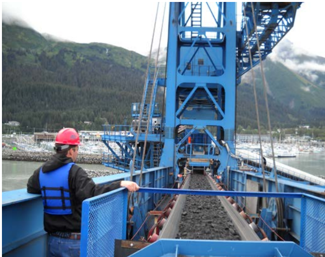
With its slide-in/slide-out cradles and external wear liner, the EVO® Conveyor Architecture simplifies maintenance.
