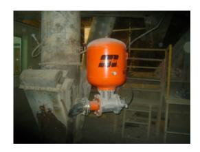
The air cannon combines a fast-acting, high-flow valve with a pressure vessel (tank). It performs work when compressed air (or some other inert gas) in the tank is suddenly released by the valve and directed through a nozzle, which is strategically positioned in the tower, duct, cyclone or other location. Often installed in a series and precisely sequenced for maximum effect, the network can be timed to best suit individual process conditions or material characteristics.
