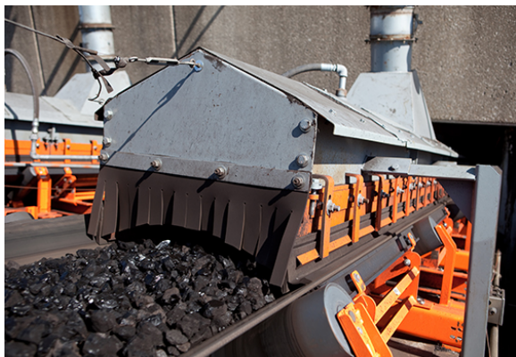
The EVO® Chute Wall System incorporates a stilling zone with staggered dust curtains to minimize airborne dust.
