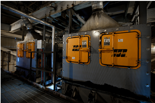
Engineered chutes employ special geometries for ease of installation with maintenance doors for easy access.
