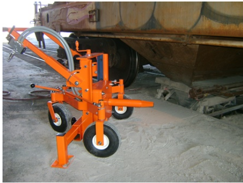
The Martin® Railcar Opener improves unloading efficiency and speed, without gang tactics, stoop labor or excessive noise.
