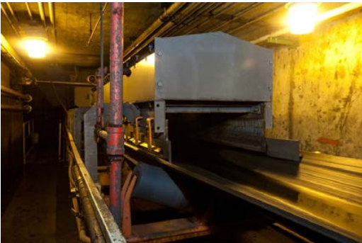
Installed at the bottom of the loading zone skirtboard, Martin® Double ApronSeal™ Skirting employs two wear surfaces on each sealing strip.
