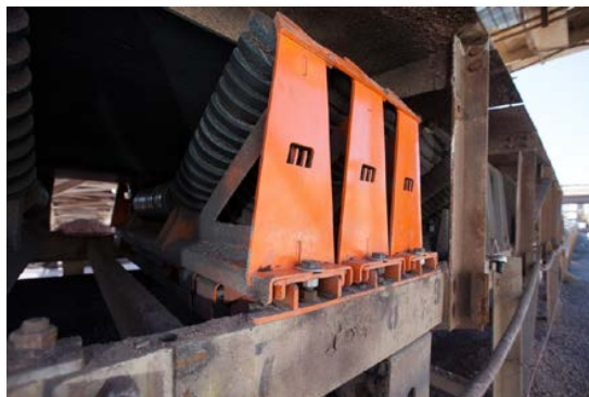
Elastomer bar suspension allows for defined vertical travel, absorbing shocks from impact maximizing the life of the belt support structure and rolling components.
