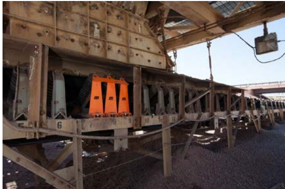
EVO® High Speed Roller Cradle is designed and engineered for high speed/high tonnage belts.
