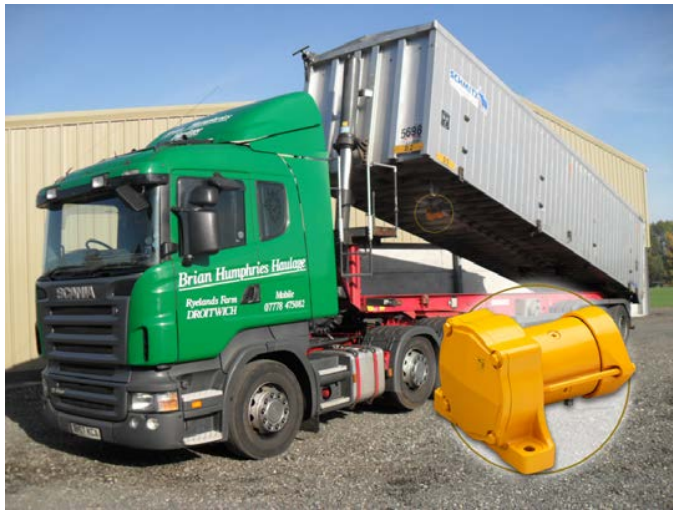
Brian Humphries Haulage is cutting its tipping time in half by using a high-performance 24V truck vibrator to more efficiently empty dump beds.
