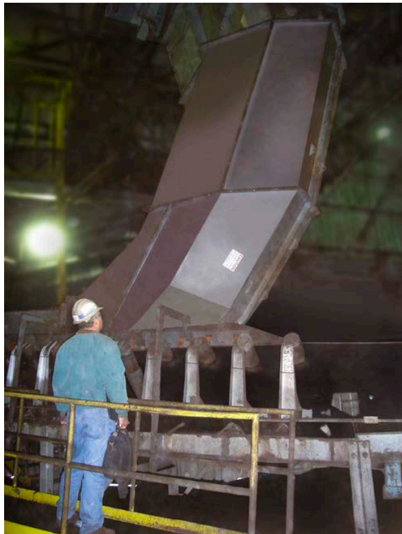
Engineered specifically for the Superior terminal, the Martin® Inertial Flow™ Transfers have minimized spillage and reduced belt abrasion.
