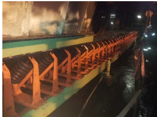
Positioned between support cradles, the Trac-Mount™ Idler frames deliver proper belt carriage to stabilize the load and improve sealing, yet they can be serviced by a single worker.
