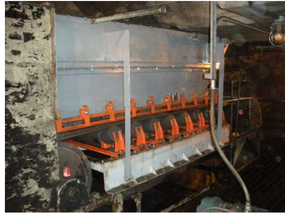
NIPSCO after: The EVO™ External Wear Liner is designed to remove the material burden from the dust containment system, diverting the bulk of the load away from the sealing components and extending their service life.
