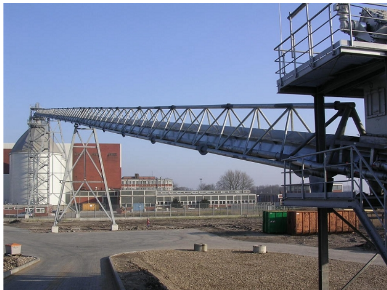
Air-supported conveyors eliminate the carrying-side idlers used on conventional design and are fully-enclosed to eliminate the the escape of fugitive materials.
