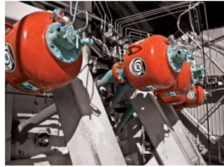
New air cannon valves from Martin Engineering produce about twice the blast force of the previous valve generation, from approximately ½ half the compressed air volume.
