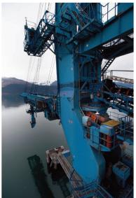
One of the worst problems was the shiploader itself. Constructed in a less environmentally sensitive era, coal dust clouds garnered negative attention that threatened the community's acceptance of the entire facility. Additionally, the malfunctioning shiploader's slow throughput extended coal loading times.
