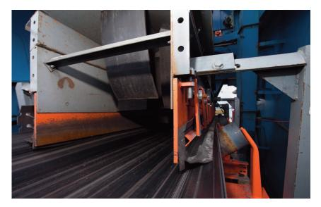
The external wear liner of the EVO system is hung on the outside of the skirtboard, to simplify installation, inspection and maintenance, while providing effective sealing at the belt edge.
