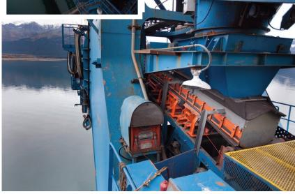
The loading zone on the boom conveyor was recently upgraded with new components from Martin Engineering's EVO conveyor architecture, including a hood-and-spoon chute and modular belt support cradles.
